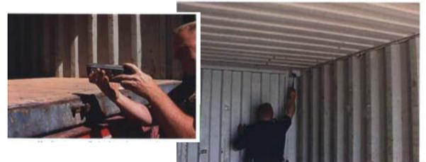
**i** Look for different wall colors and blocks that are too close to the vents. Use a tool to tap front wall – you should hear a hollow, metal sound.
