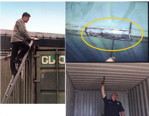
**i** Any weld repairs on the inside must be also be visible on the outside. Watch for unusual welding or repair on support beams. False compartments are common in ceilings, beams, floors, doors, and the front wall.
